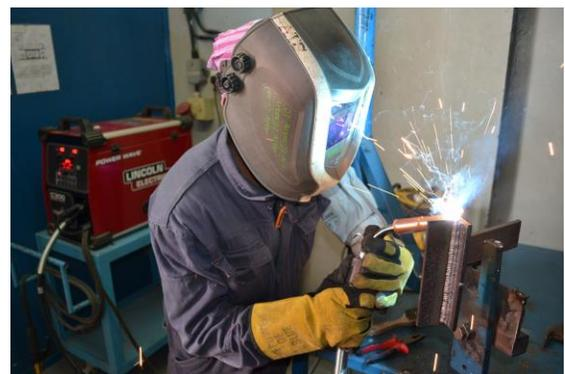
PPE – Proper PPE varies with the type of welding. Make sure you use correct eye protection, gloves, and appropriate clothing when operating this tool. Others adjacent to the welding area need to be notified of the activity allowing them to put on proper PPE or to leave the area.
