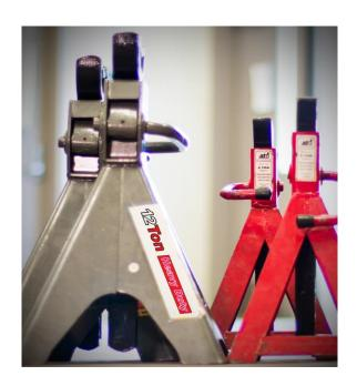
If you are using an older, unmarked jack stand, take the time to look up the stand's load rating specifications and then mark it visibly and permanently on the stand. If you cannot verify a jack stand's load rating, pull it from service (Tag Out) and replace it with a one stamped with the proper load rating.
