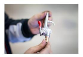
**Hazards.** Filings, chips, shavings, particles of metal, and other materials can become projectiles when compressed air is used for cleaning purposes.
