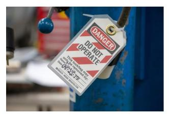
An example would be a bench grinder in need of a new wheel. To safely replace it, you should unplug it from the power source and tag the plug. If it is hard wired, turn off the breaker at the panel and lock the breaker in the off position. Can't lock it? Then tag the breaker so that someone will not turn the breaker on. The idea is to make it clear that someone is working or equipment in need of repair.
