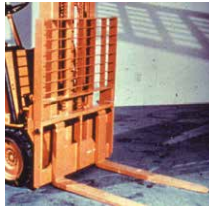
A backrest extension keeps the load from falling rearward.
