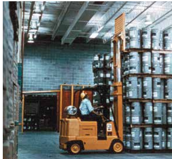
Internal combustion engine forklifts can cause carbon monoxide poisoning when used indoors if the engine is not kept tuned and the area well ventilated.
